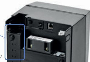
Built-in power supply
